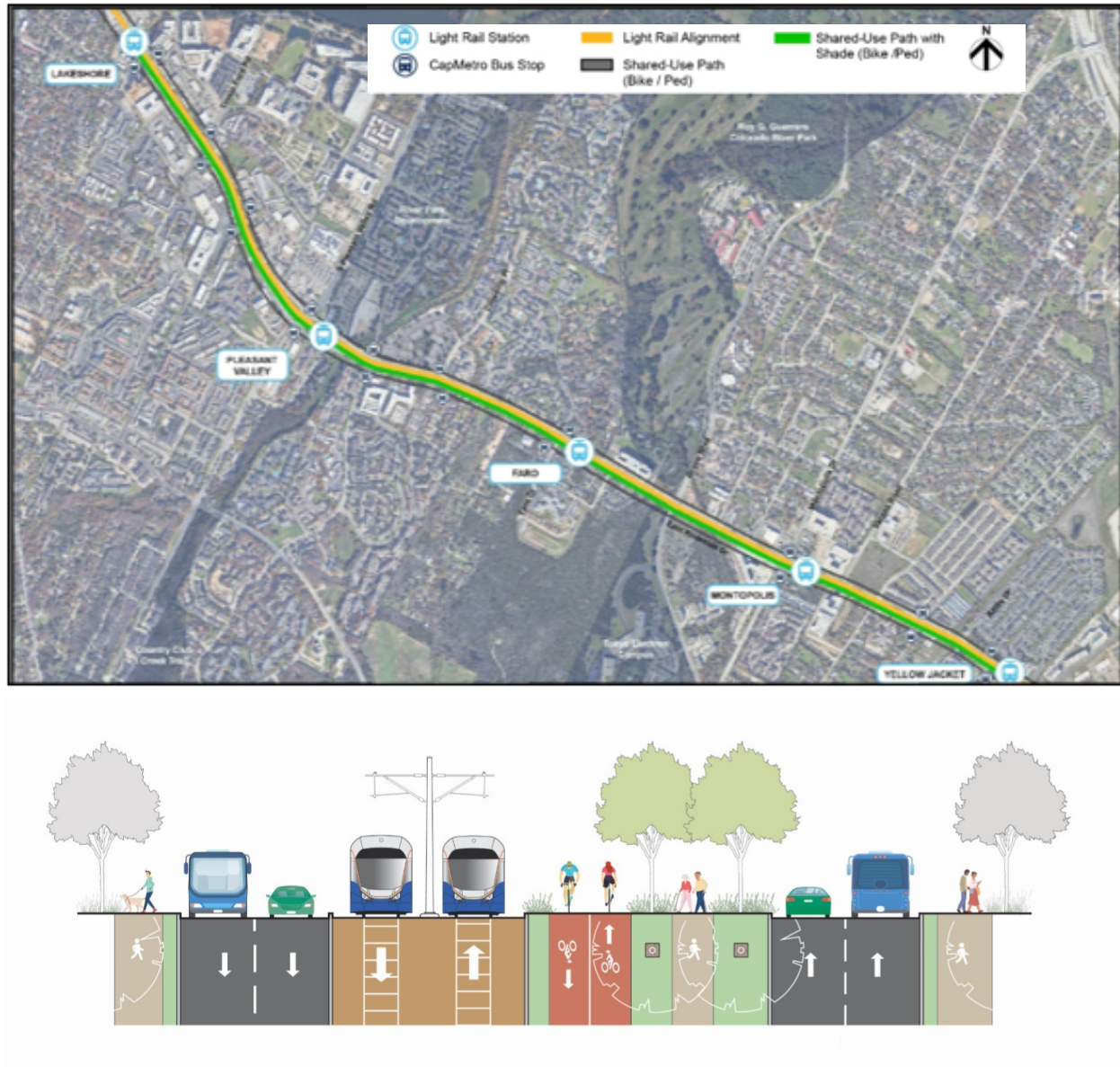
Figure 7-10: Cross Section View of Center-Running Bike/Pedestrian and Shade Tree Facilities on East Riverside Design Option
