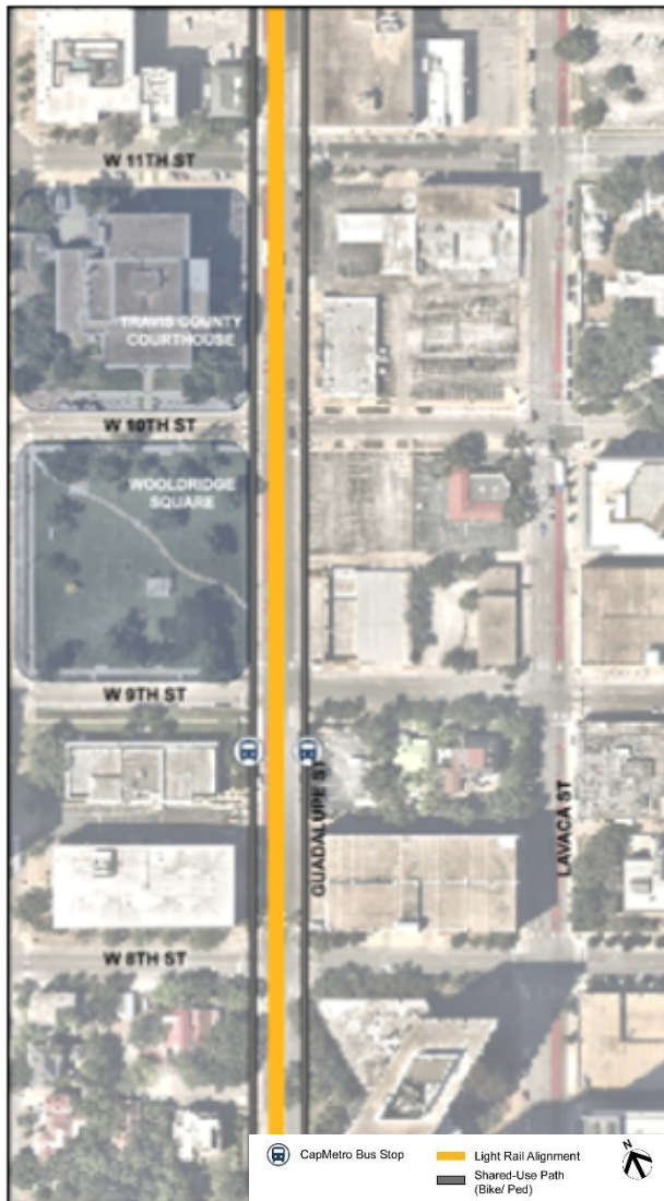
Figure 7-1: Build Alternative near Wooldridge Square
