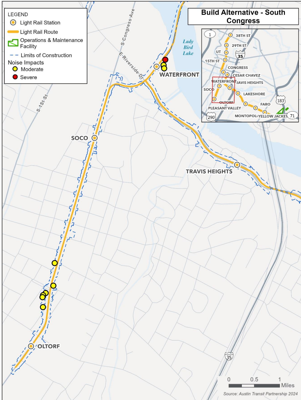
Figure 12: Build Alternative Noise Impacts – South Congress
